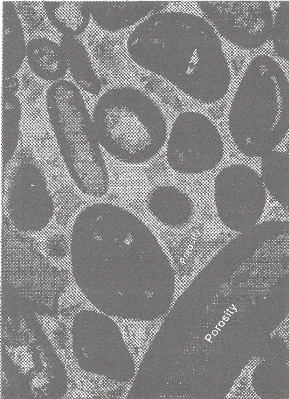
Figure 3. Thin section of lower Pettet (Frost "A") depicting intergranular and intragranular porosity.
