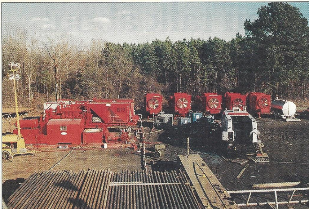
Each one of the five, three-stage, positive-displacement air boosters on the Pirkle 2 location was capable of 1,500 scfm of output capacity (Fig. 4).
